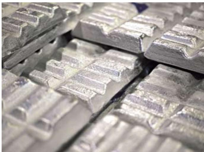
AMG – typical master alloys in ingot form
