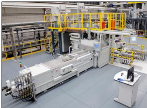
Vacuum Turbine Blade Coating EB/PVD Production Systems, Type SL XXL
