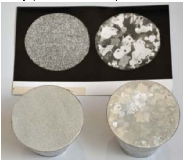
1 Cast aluminium samples before (right) and after (left) the addition of TiBAI™ 5/1 grain refiner.
